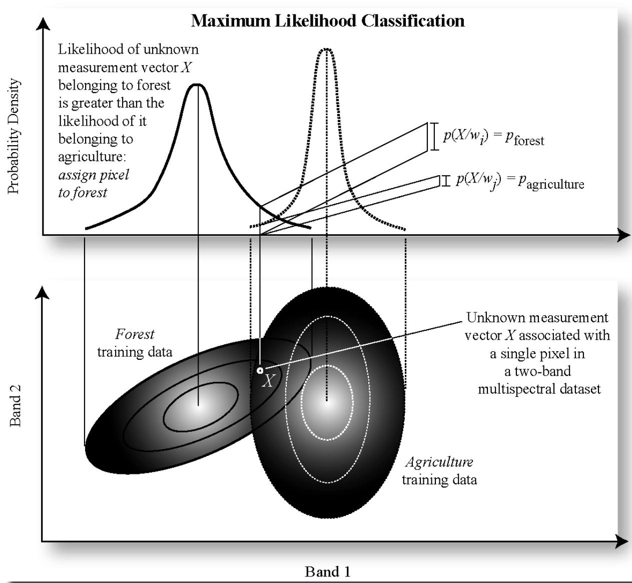
In this case, pixel  $X$  would be assigned to forest because the probability density of unknown measurement vector  $X$  is greater for forest than for agriculture.
