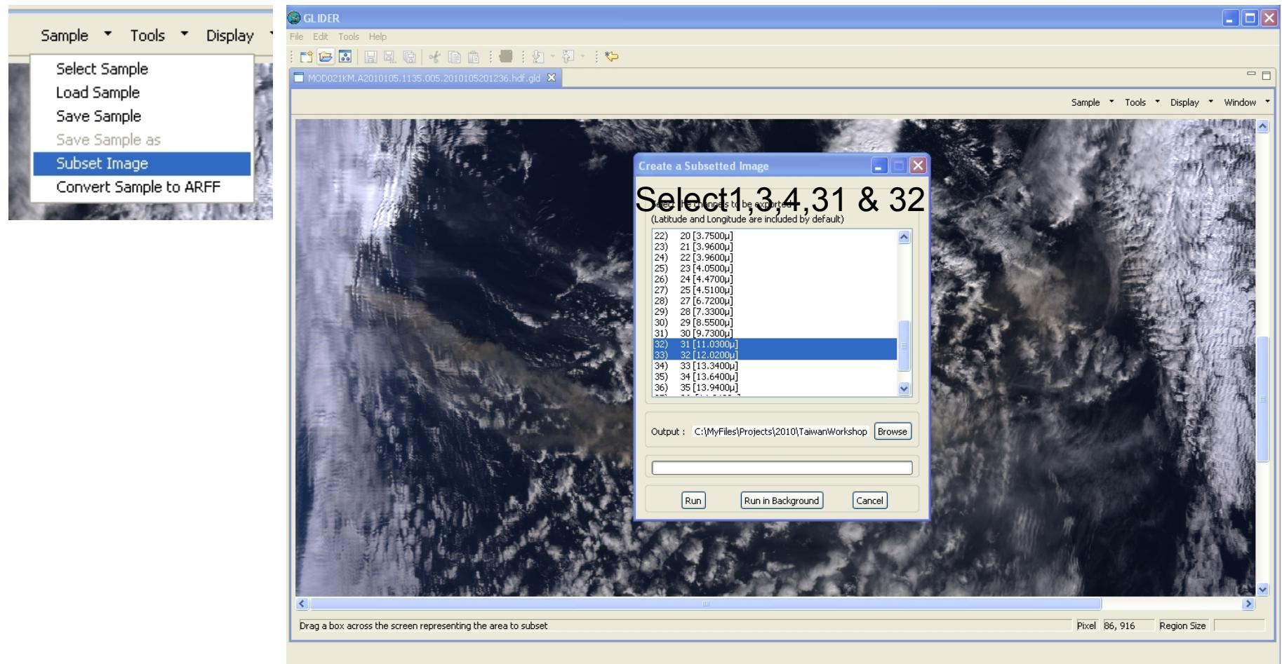
Select an area within the Image View, then select Bands, provide output filename (subset.gld) and hit Run button. Go to Project View and load subset.gld in Image View
