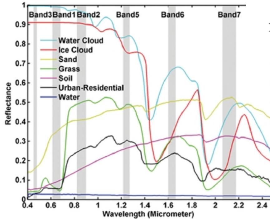
$$\text{NDDI} = (\rho_{2.13\mu\text{m}} - \rho_{0.469\mu\text{m}})/(\rho_{2.13\mu\text{m}} + \rho_{0.469\mu\text{m}}) \quad (1)$$
