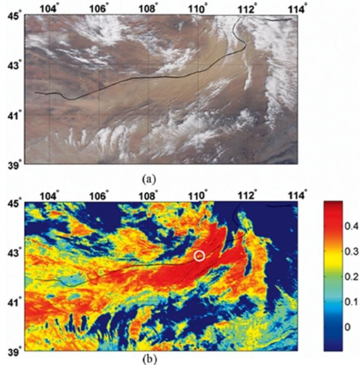
Fig. 3. (a) Terra MODIS true-color image (3:40 UTC, March 27, 2004) shows Asian dust storm over Northern China and Southern Mongolian regions. (b) Terra MODIS NDDI image shows the clouds and dust storms. The cloud and dust storm can be easily identified (for cloud NDDI  $< 0.0$  and for dust storm NDDI  $> 0.28$ ).
